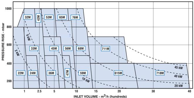
Notes: 1. Pressure ratings based on inlet air at standard pressure of 1013 mba, standard temperature of 20°C. 2. Universal RAI blowers may also be used on vacuum service. For performance charts, contact sales office.
