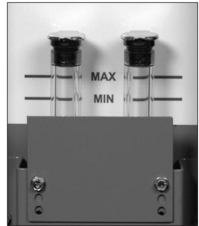
Oil fill level site glass.
